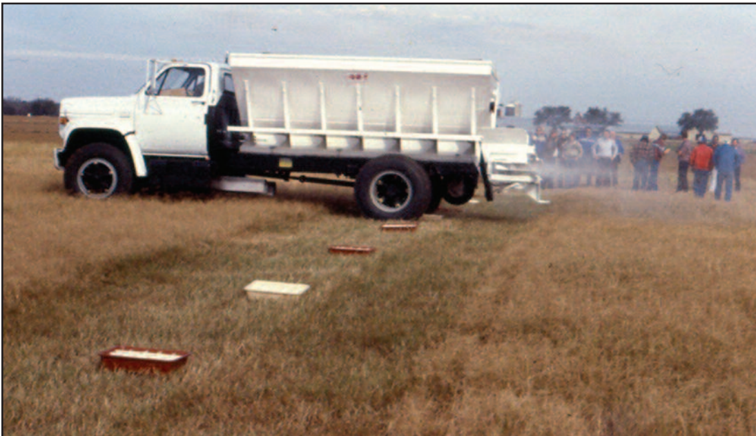
Lack of fertilizer spreader calibration can result in uneven nutrient distribution that leads to "streaky" fields.
