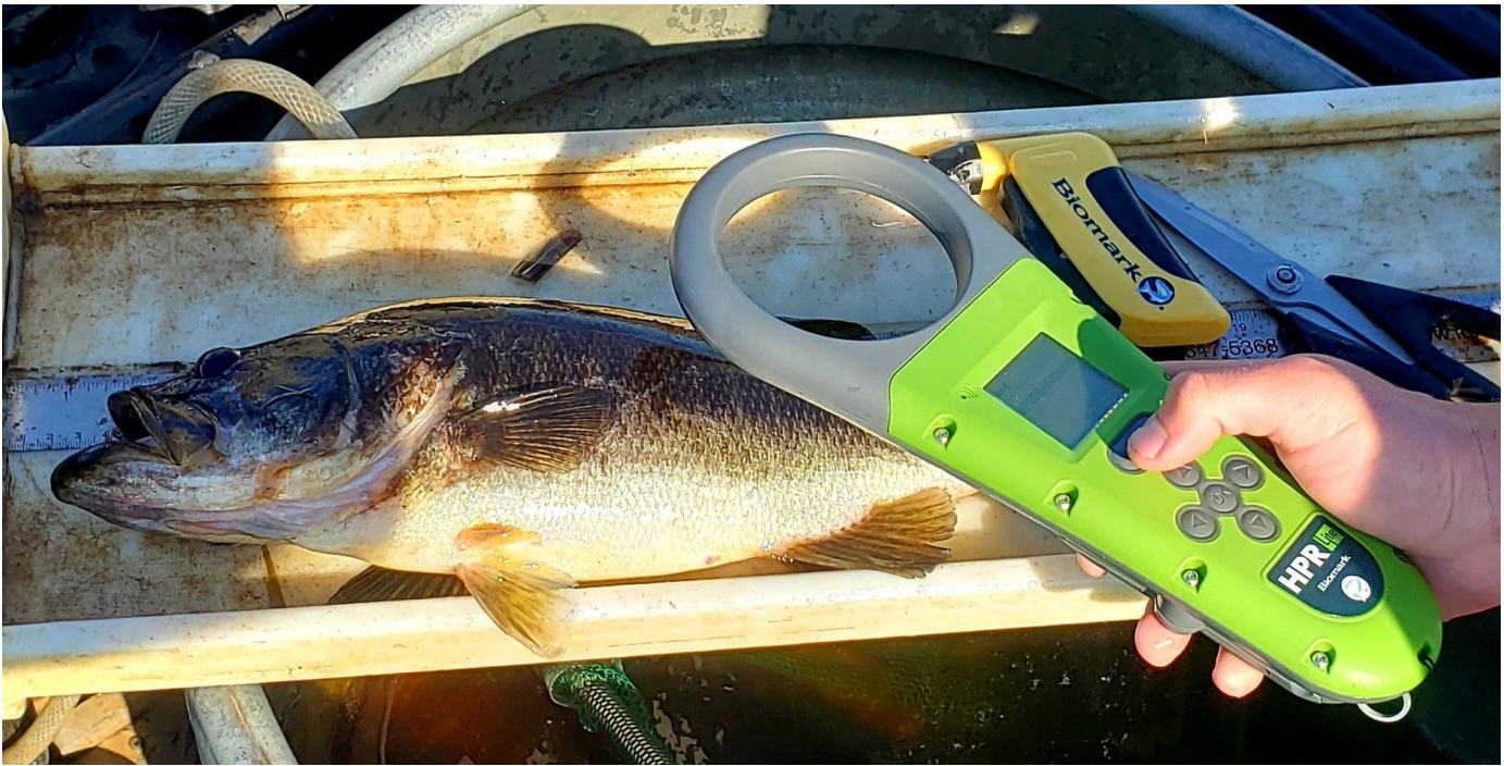
After the PIT Tag (Passive Integrated Transponder) is inserted, the fish must be scanned, and the number recorded and assigned to that individual.
