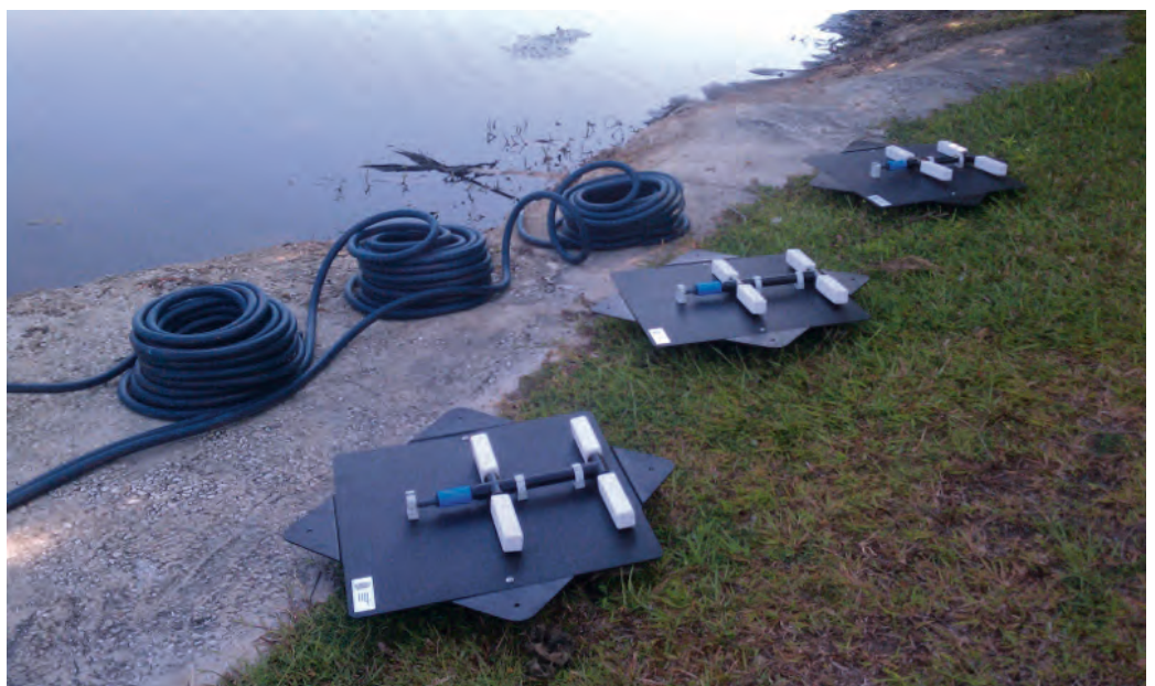
Bottom aeration is a big help in preventing fish kills. If conditions get too poor, a fish kill may still happen, but its severity may be less and you will have fewer of them.
